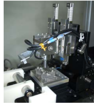
Fig. 1. A specially-designed scratch tester for evaluating CrAl-coated cladding layer on conventional Zr-based alloys.
